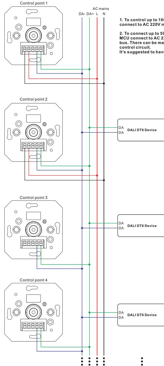
1. To control up to 100 ECG with the setup(Figure 2), there is 2 MCUs connect to AC 220V mains.
