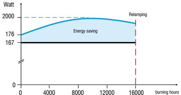
Fig. 1 - System power at inductive ballasts
