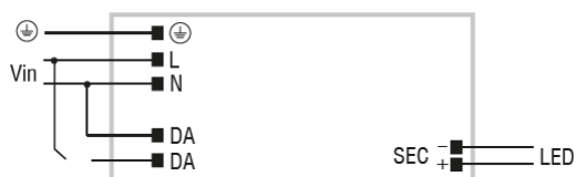
PUSH SWITCH diagram Collegamento PUSH SWITCH
