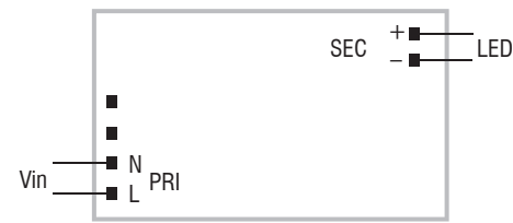
CASAMBI Wireless diagram Collegamento Wireless CASAMBI
