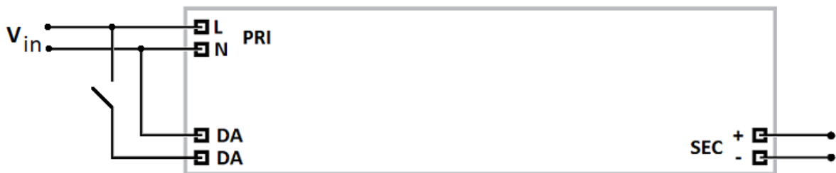
PUSH SWITCH connection diagram Schema di collegamento PUSH SWITCH
