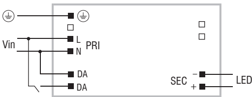
PUSH SWITCH diagram - Collegamento PUSH SWITCH
